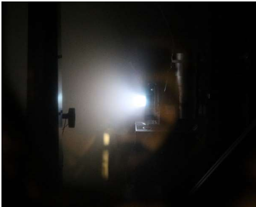
Fig.1: Left) ECRA thruster placed on the thrust balance and running at JLU's JUMBO facility. Right) Comparison of the measured thrust of the RIT 4 and the theoretical thrust
